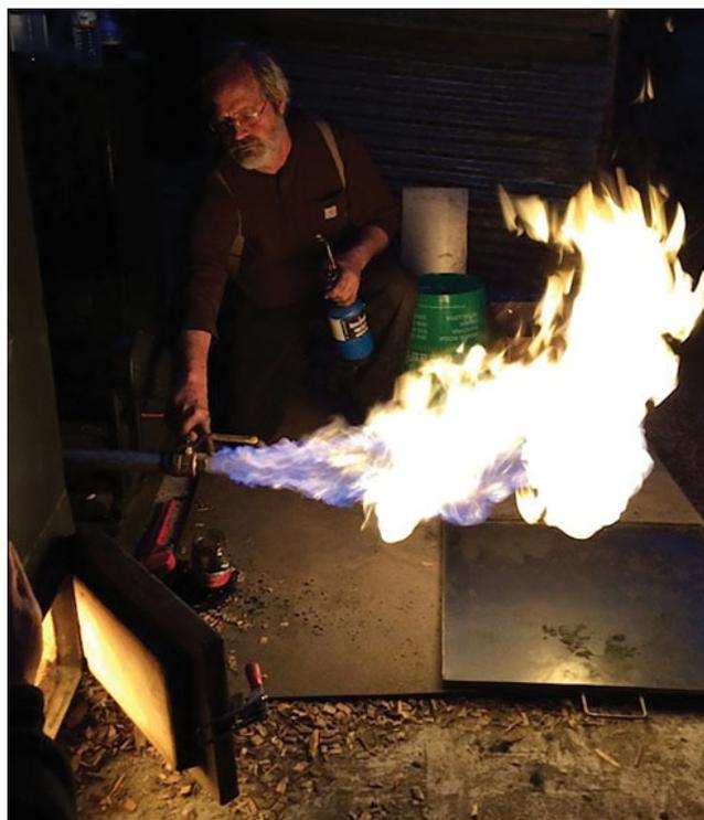
**Figure 2: Bob Wells adjusts the flare while operating his biochar retort. A retort is an airtight vessel in which substances are heated for a chemical reaction, producing gaseous products to be collected for further processing.**
